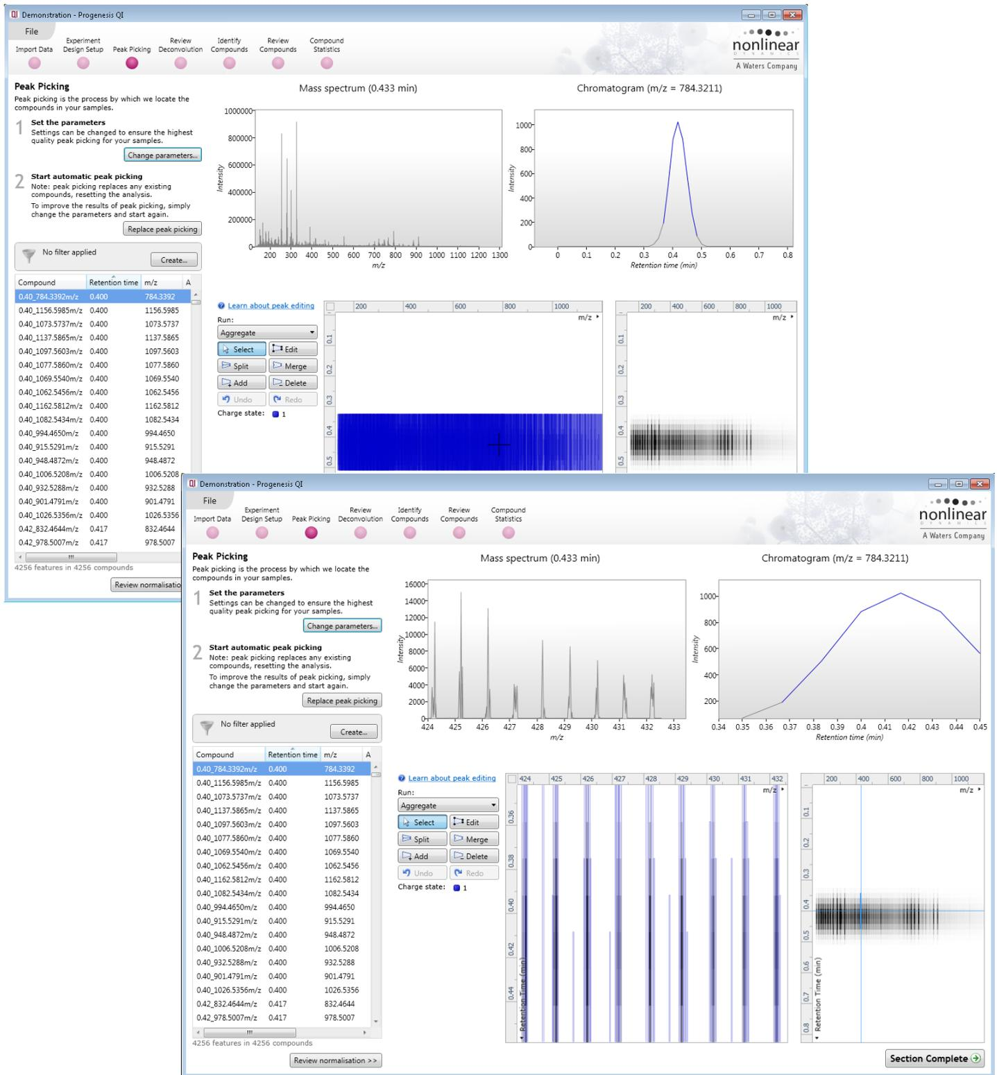
**Figure 13:** At **Peak Picking** the detected m/z profile is visible. The profile will potentially appear quite crowded (back panel), but on zooming in (front panel) separate ions can be distinguished.
